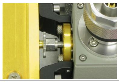
Figure 6-4. Installing WG Flange with Limited DUT Space
