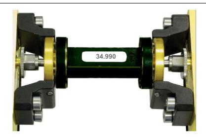
Figure 6-8. Two Port Alignment with DUT
