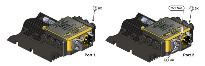
Figure 6-7. Port 1 and Port 2 Alignment
